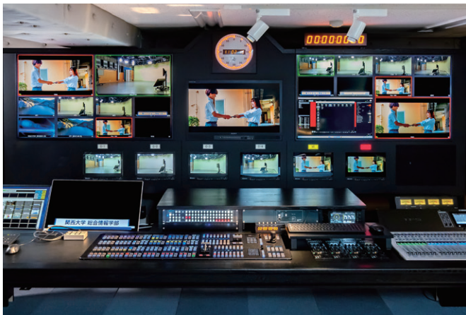
▲ KAIROS' control panel (center of switcher table) and two multi-viewers (on monitor shelf) can be customized to fit any layout.
