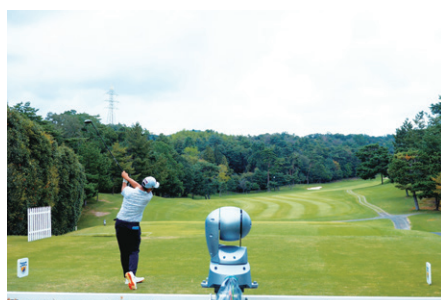
▲ High-quality PTZ camera installed at the first hole to capture opening tee shots
