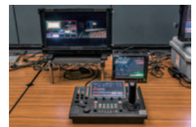
▲ The AW-RP150GJ used for VE. This was used to adjust the brightness and color of the footage from the four AG-CX350s and two AW-UE150W/Ks in the hall.
