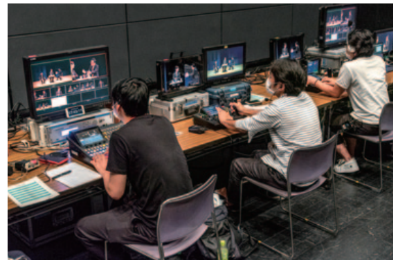
▲ The film base during the show. From the front: the AV-UHS500, the AW-RP150GJ (to control the AW-UE150W/Ks) and the AW-RP150GJ (for VE)
