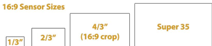
1/3" camera, and that offers the benefits of a 1/3" camera's integrated power zoom lens, autofocus and image stabilization, but which also preserves the ability to create shallow depth of field similar to the Super 35 camcorder. The DVX200 uses a Four Thirds sensor, which is approximately four times larger than the 2/3" sensor, nearly 16x larger than the 1/3" sensor, and is reasonably close in size to a Super 35 sensor.
