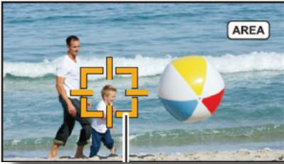
**AREA mode:** You can specify what area on the screen you want the autofocus system to concentrate on (and, by default, you're telling the system to ignore the rest of the screen!) Not only can you specify the area, but you can also choose how large of an area to focus on (small, medium, or large). This feature is quite useful for sit-down interviews or for shots where you are consistently framing your subject into a certain section of the display.
