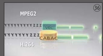
Context-Adaptive means "adapting to surrounding circumstances." By using this Context-Adaptive technique in arithmetic coding, CABAC can achieve ideal entropy encoding efficiency close to the theoretical limit.
