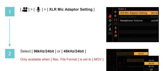
When the DMW-XLR1\* is attached, audio is down-converted to a format suitable for the connected HDMI external device before being output.
