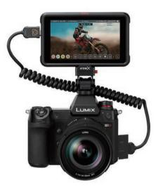
Connect the camera and the external recorder with an HDMI cable, and turn them on.
