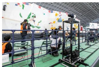
▲ The AW-UE150K on a motorized dolly was connected to the relay booth via a 50m fiber-optic cable for a simple, labor-saving setup.
