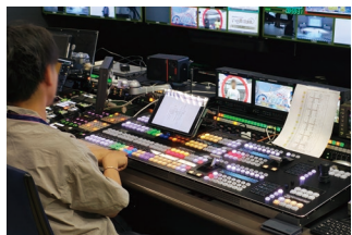
▲ Kairos Control panel at Kansai Television Co. used for remote production
