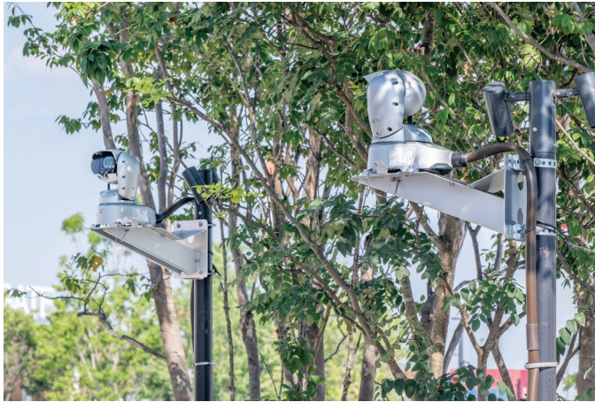
▲ Two AW-UR100 PTZ cameras capture fabric panel movements while blending into the environment
