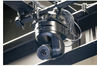
▲ AW-UE160K camera mounted on the ceiling of Zone 2 to capture visitor activity
