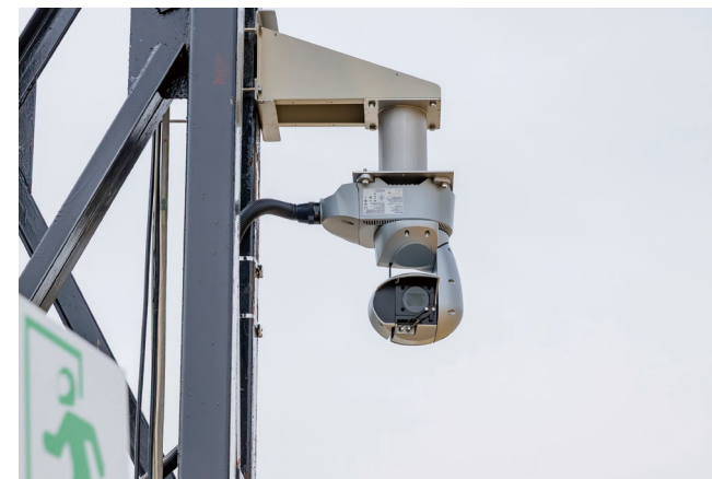
▲ IP65-rated AW-UR100 ensures reliable operation even in harsh weather, with a built-in lens wiper for rainy-day shooting.
