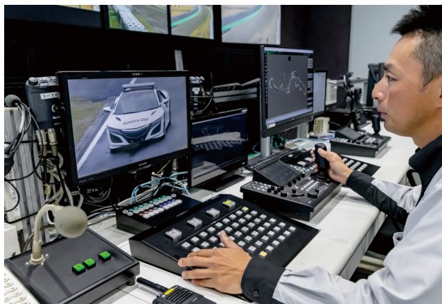
▲ AW-UR100 camera operated with a custom switcher and the AW-RP150GJ Remote Camera Controller.
