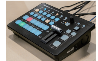
▲ Using the AV-HSW10 switcher to manage transitions between scenes and other video sources.
