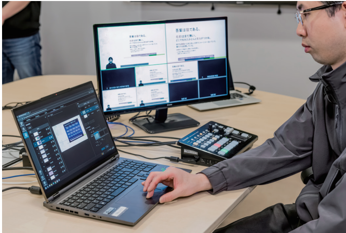
▲ Video Mixer installed on a laptop PC receives feeds from one camera and presentation visuals from another PC.
