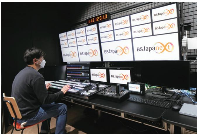
▲ T4 control room equipped with KAIROS, where each user can freely change the layouts of the two multi-view screens.
