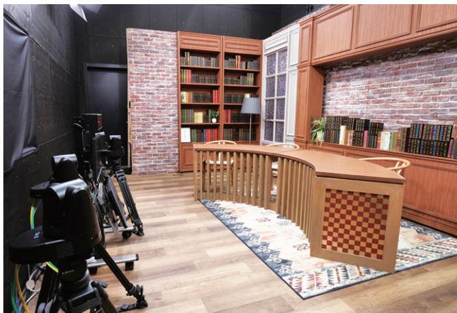
▲ T4 studio with four 4K Integrated Cameras (AW-UE100K) for shooting in 4K and cropping in 2K, enabling three to four images per camera.
