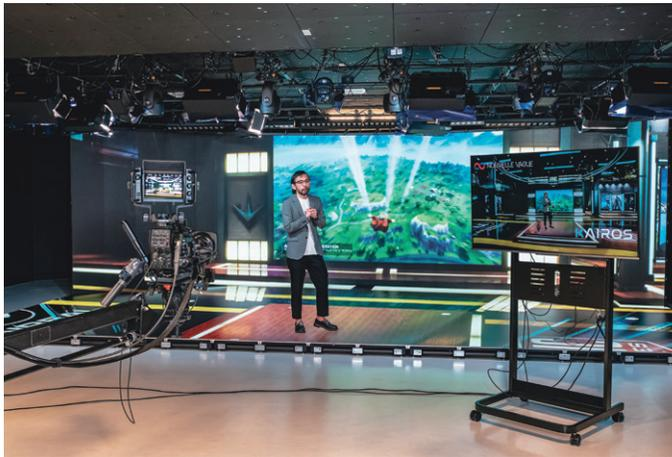
▲ Mixed-reality studio equipped for in-camera VFX. Computer graphics and images projected on a large, high-definition LED screen are combined in real time with performers in the foreground in a fusion of virtual and real worlds.
