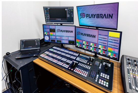
▲ KAIROS control panel with two multi-view screens positioned directly in front, Kairos Creator PC on operator's left for convenient instant access.
