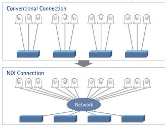
With NDI Connection, a control room or multiple control rooms are all connected. All video sources are available to all video destinations without a separate cable. Simpler to connect, easier to deploy, offering even more production creativity!
