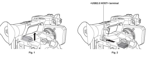
1 Open the <USB2.0 HOST> terminal cover on the top-back side. (Fig. 1)
