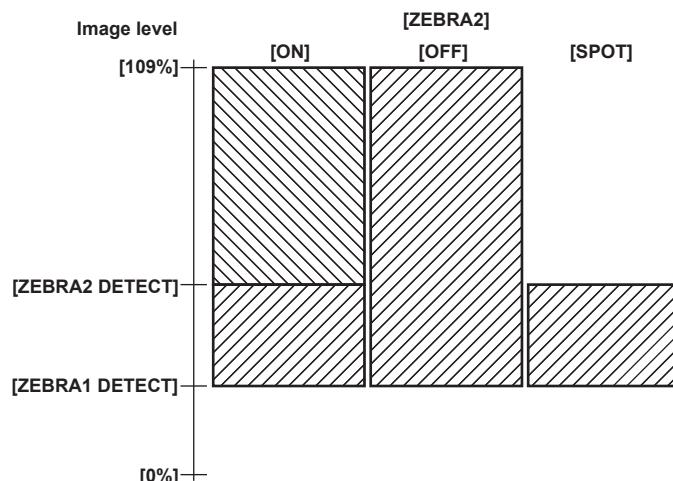
When displaying the zebra pattern in the video output from <SDI OUT1> and <SDI OUT2> terminals, perform setting in the [VIDEO OUT/LCD/VF] menu → [SDI OUT1]/[SDI OUT2] → [SDI OUT ZEBRA].
