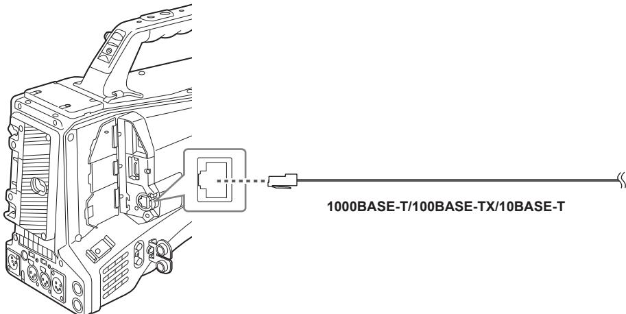
**1** Insert the LAN cable into the <LAN> terminal.
