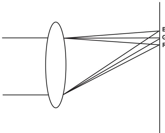
“Chromatic aberration” here refers to zoom factor chromatic aberration. Zoom factor chromatic aberration occurs since the diffraction ratio of a lens differs according to red (R)/green (G)/blue (B). Chromatic aberration on the lens itself is compensated for, but still remains in the periphery, in particular. Also, this chromatic aberration occurs on zoom lens due to a complex relationship between zoom ratio, aperture and focal distance. In image terms, this is registration error.
