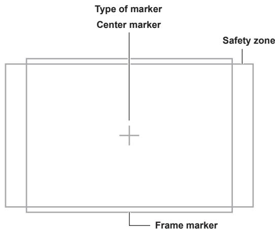
Pushing the <MARKER SEL>/<MODE CHECK> switch on the camera towards the <MKR> side switches the marker on the viewfinder in the order of [A] marker, [B] marker, and no display.
