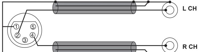
Do not use the cable where the pin 3, pin 5 and pin 1 are connected. Doing so may result in a malfunction.
