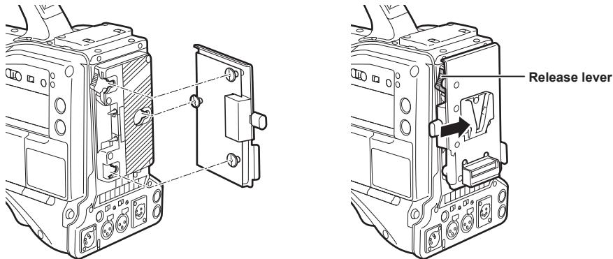
**1** Mount the V-mount type battery plate.
