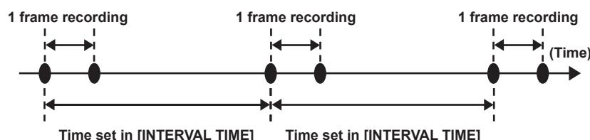
**1 Select the [RECORDING] menu → [REC FUNCTION] → [REC MODE] → [INTERVAL].**
