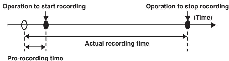
The pre-recording time varies depending on the setting of the [SYSTEM] menu → [FILE FORMAT]/[REC FORMAT].
