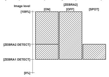
To display the zebra patterns in the video of the monitor output terminal (<GENLOCK IN/VIDEO OUT>), set in the main menu  $\rightarrow$  [OUTPUT SEL]  $\rightarrow$  [VIDEO OUT ZEBRA].
