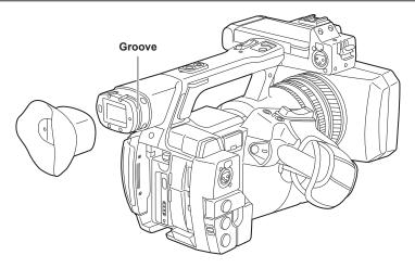
1 Attach the eye cup by aligning the groove on the attaching part of the eye cup with the inner ridge of the eye cup.
