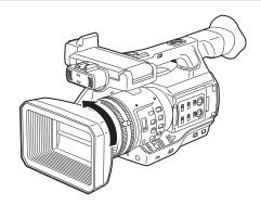
1 Rotate the lens hood counter-clockwise.
