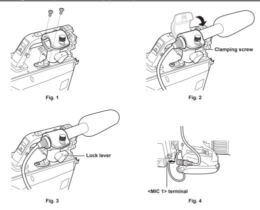
Remove the screws on the microphone holder mounting position and mount the microphone holder AJ-MH800G (optional). (Fig. 1)
