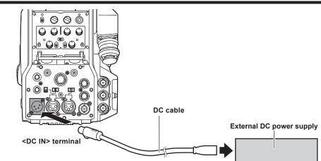
1 Connect the external DC power supply to the <DC IN> terminal on the camera.
