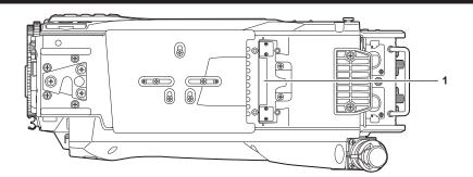
1 Build-up terminal Used to connect the Build-up Unit AK-HBU500G (optional).
