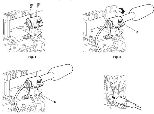
1 Remove the screws at the microphone holder mounting position and attach the microphone holder AJ-MH800G (optional). (Fig. 1)
