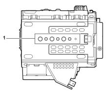
1 Shoulder mount module/tripod mounting holes For attaching the shoulder mount module or a tripod.
