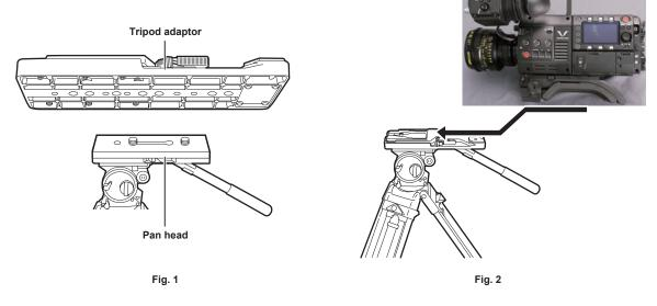
1 Mount the tripod adaptor on the tripod. (Fig. 1)
