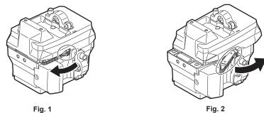
1 While raising the lock knob (red) of the recording extension module release lever (Fig. 1), pull the recording extension module release lever. (Fig. 2)
