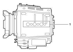
1 Shoulder mount module/tripod mounting holes
