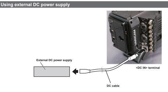
**1** Connect the external DC power supply to the <DC IN> terminal of the camera.
