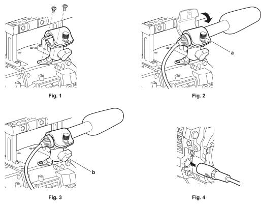
**1** Remove the screws at the microphone holder mounting position and attach the microphone holder AJ-MH800G (optional). (Fig. 1)
