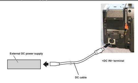
**1** Connect the external DC power supply to the <DC IN> terminal of the camera extension module.
