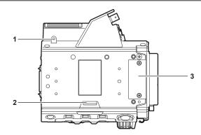
1 Mounting hole for control panel mounting part
