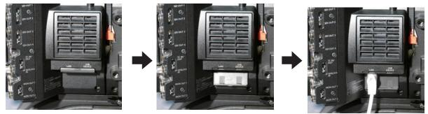
**1** Connect the LAN cable to the <LAN> terminal on the right side.
