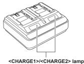
The <CHARGE1>/<CHARGE2> lamp (charging lamp) of the supplied battery charger indicates the charging status as follows.
