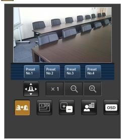
When this button is pressed, the buttons for selecting the preset positions are displayed on the screen.
