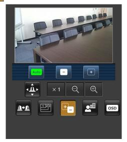
When this button is pressed, the buttons for performing the iris operations are displayed on the screen.
