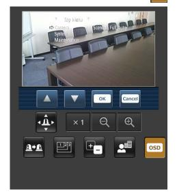
When this button is pressed, the buttons for performing the camera menu operations are displayed on the screen. At the same time, the camera menus are also displayed on the monitor images of the unit.
