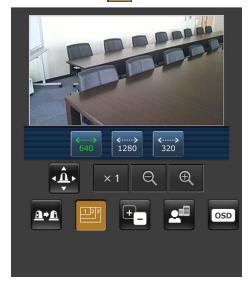
When this button is pressed, the buttons for selecting the resolution are displayed on the screen.
