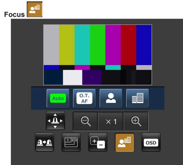
When this button is pressed, the buttons for performing the focusing operations are displayed on the screen.
