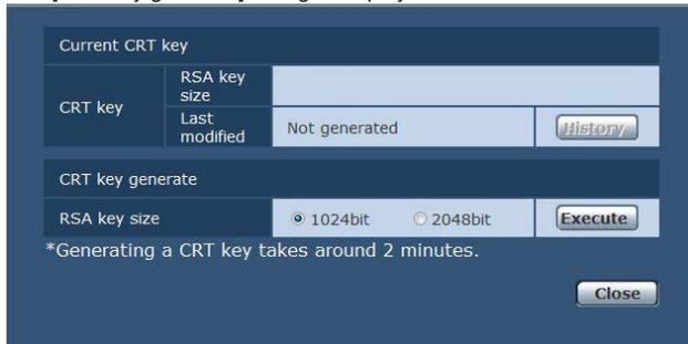
**2. The size of the generated CRT key is selected from [1024bit] / [2048bit] in [CRT key generate] – [RSA key size].**
