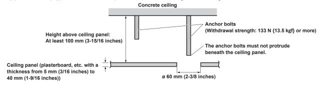
1. Refer to the Operating Instructions of the WV-Q105A direct ceiling mount bracket, and attach the WV-Q105A as well as the drop-prevention wire angle and drop-prevention wire supplied with the WV-Q105A to the anchor bolts.
