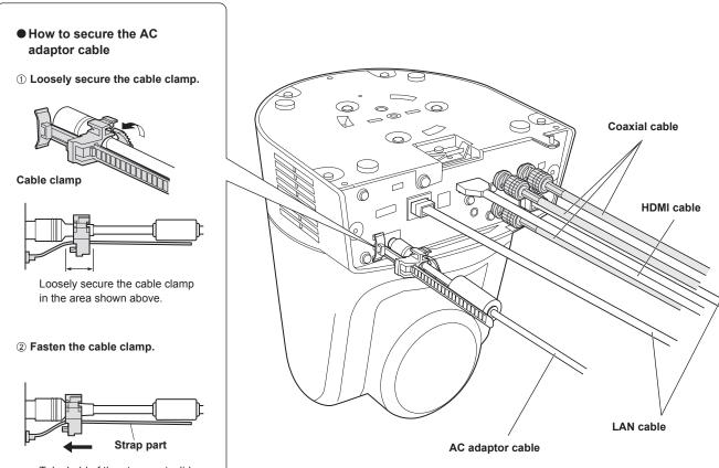
Take hold of the strap part, slide the cable clamp until it stops moving, and then secure it tightly.
