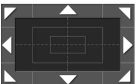
To adjust the image in the horizontal or vertical direction (panning or tilting), left-click the pad and the buttons.</p> <p>It is possible to operate with the central grid pattern in the dragged state, with the speed of the pan/tilt increasing as it approaches the outside of the pad.</p>
