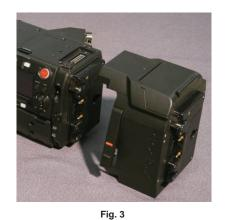
1 Slide the stopper on the release lever on the V-RAW recorder, and pull up the release lever. (Fig. 1, Fig. 2) The V-RAW recorder will lift.
